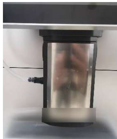
BEVERAGE OUTLET ASSEMBLY — REMOVE FOR CLEANING AS SHOWN.
