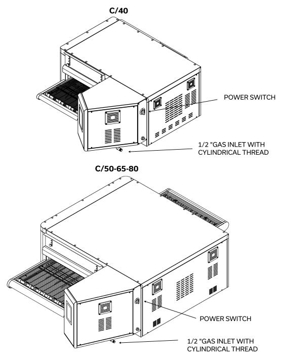
Natural gas is connected to the network.
