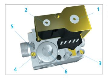
To adjust the outlet pressure, loosen the screw at position number 4 and connect a differential pressure meter.
